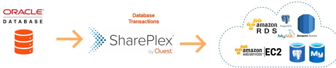
Fig 2: Hybrid cloud infrastructure showing Oracle data replication to MySQL and PostgreSQL targets in AWS
